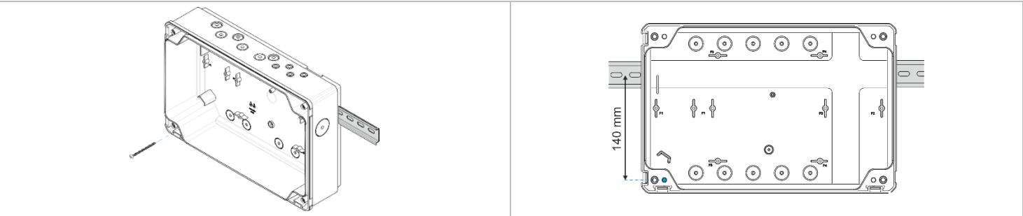
XER can be mounted on DIN rail and fixed using 1 screw (type: D4.5mm x L55mm)
