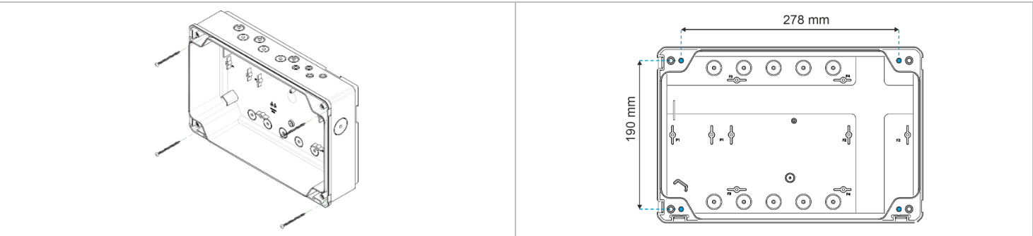
XER can be mounted on a wall and fixed using up to 4 screws (type: D4.5mm x L55mm)
